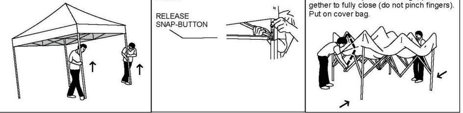
2 Release auto slider at each corner by pushing Snap-Button to release pressure on slider. Repeat on all four corners.
